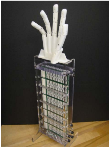
Fig. 2 Picture of the Robotic Hand Prototype used to design and test the multi-axis array segmentation architecture
